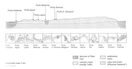
Geologic cross section below the Aurelian Wall. Gates most heavily damaged by earthquakes are those located on alluvium rather than rock.
