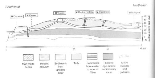
You get an idea of the remarkably thick layer of man-made debris that covers the city by studying this geologic cross section along the Metropolitana B (subway) between stations at Piazza Bologna and the Colosseum. For example, the ravine near Cavour station is filled with 20 meters (66 feet) of debris. The illustration is exaggerated vertically to show the relations between geologic units (measured in meters above sea level).
