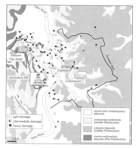
This map showing the basic geology of the historical center of Rome indicates those monuments that have required repair and restoration after earthquakes. The most heavily damaged areas are those on the Tiber River floodplain, where the sites are underlain by thick deposits of river sands and gravels.
