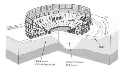
As you can see from this diagram of the Colosseum (Flavian Amphitheater), the north side of the Colosseum (to the left), which is underlain by marine sedimentary rocks and tuff, suffered only light damage during the earthquakes of the centuries. The southern side, overlying an ancient creek filled with poorly consolidated sediment, was severely damaged by excessive ground acceleration within the alluvium during large earthquakes.
